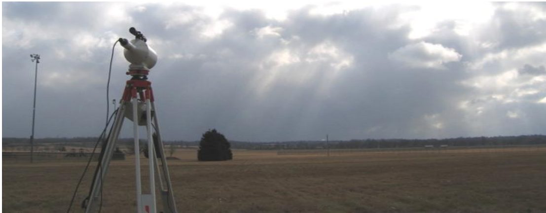
Figure 14. Scintillometer receiver looking down the path towards the weather station and transmitter. Path length is ~800m. Weather station placed in middle of path range.
