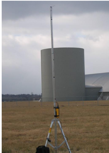
Figure 16. Thermocouple tripod station for two levels of temperature measurements, located in the middle of the BLS900 path, slightly offset, just as weather station set-up. Note lack of shading devices used this day due to overcast.
